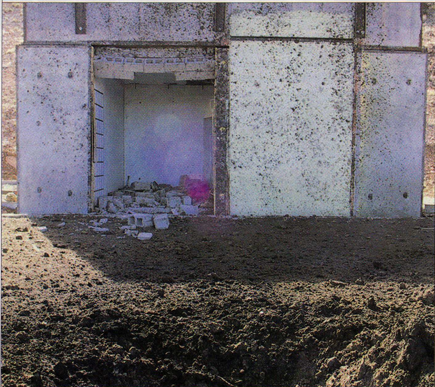
In testing sponsored by the Department of Defense, two unreinforced concrete masonry walls were constructed within a larger containment structure, with each wall being 8-ft. wide x 11-ft. high. One wall served as the control specimen (below left), and the other was retrofitted with Blastek inside and outside (above and below right). A TNT explosive blast destroyed the control wall, while the protected one remained intact.
