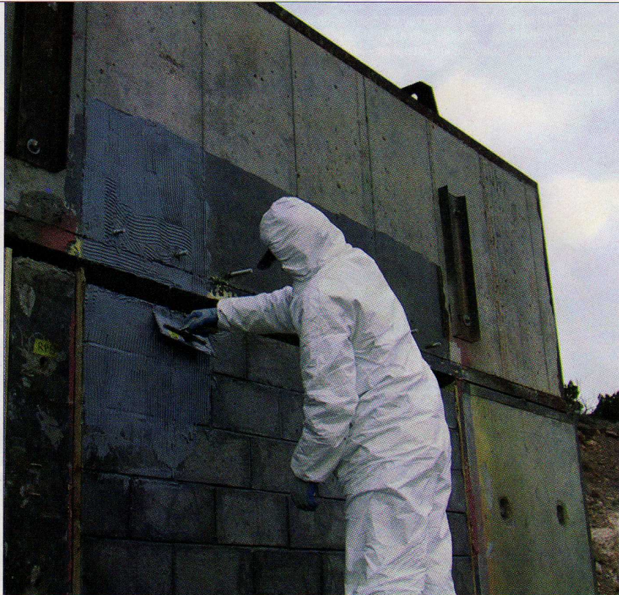
In testing sponsored by the Department of Defense, two unreinforced concrete masonry walls were constructed within a larger containment structure, with each wall being 8-ft. wide x 11-ft. high. One wall served as the control specimen (below left), and the other was retrofitted with Blastek inside and outside (above and below right). A TNT explosive blast destroyed the control wall, while the protected one remained intact.
